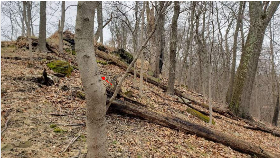
PHOTO 12: Outcrop on the western end of the site, looking east. Note: Bowed trees indicating slow movement over time
